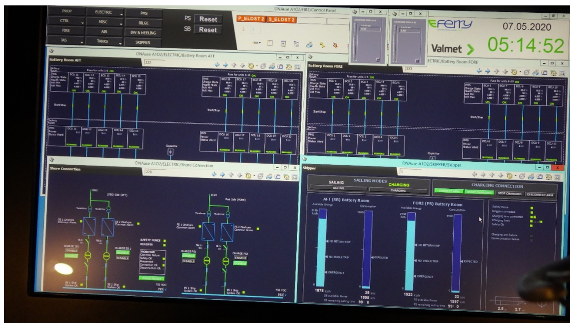
Figure 17: Available calculated battery capacity as shown to crew on bridge as of May 7, 2020, lower right corner.
